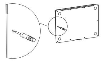
INSTALL LEDGE WHILE THE LAPTOP'S LID IS OPEN WITH THE SCREW PROVIDED
