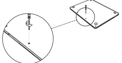
ALIGN THE "LEDGE" WITH THE SCREW HOLE AND FASTEN WITH SUPPLIED SCREW
