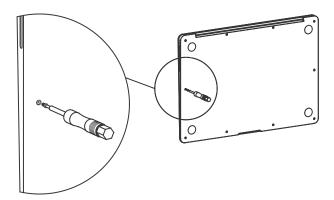
INSTALL LEDGE WHILE THE LAPTOP'S LID IS OPEN 2 WITH THE SCREW PROVIDED
