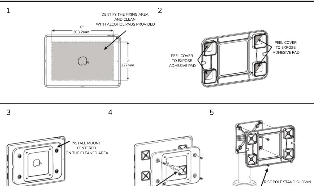
ACHIEVES FULL STRENGTH AFTER 12 HOURS REMOVE MOUNT FROM DEVICE BY REMOVING M4 PIN TORX SCREWS USING PROVIDED T-15 SCREWDRIVER INSTALL MOUNT ON ANY 100mm VESA COMPATIBLE STAND OR ARM USING PROVIDED M4x10mm PHILLIPS PAN HEAD SCREWS
